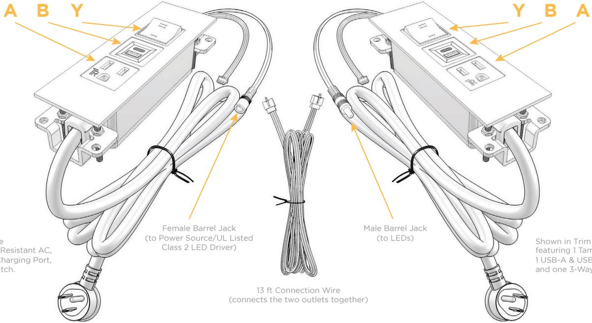
Shown in Trim Plate featuring 1 Tamper Resistant AC, 1 USB-A & USB-C Charging Port, and one 3-Way Switch.
