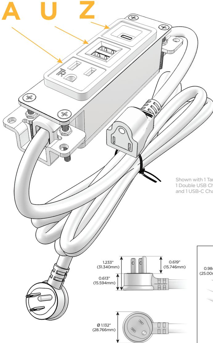
Shown with 1 Tamper Resistant AC, 1 Double USB Charging Port, and 1 USB-C Charging Port.
