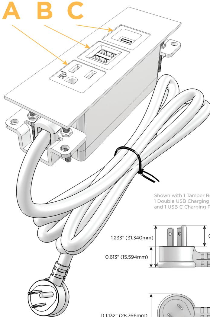
Shown with 1 Tamper Resistant AC, 1 Double USB Charging Port, and 1 USB C Charging Port.
