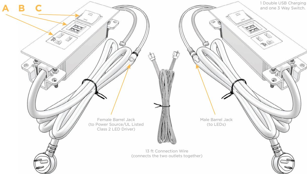
Shown with 1 Tamper Resistant AC, 1 Double USB Charging Port, and one 3 Way Switch.
