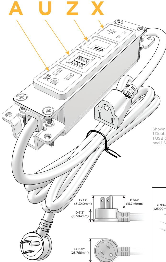
Shown with 1 Tamper Resistant AC, 1 Double USB Charging Port, 1 USB C Charging Port, and 1 Switched AC.
