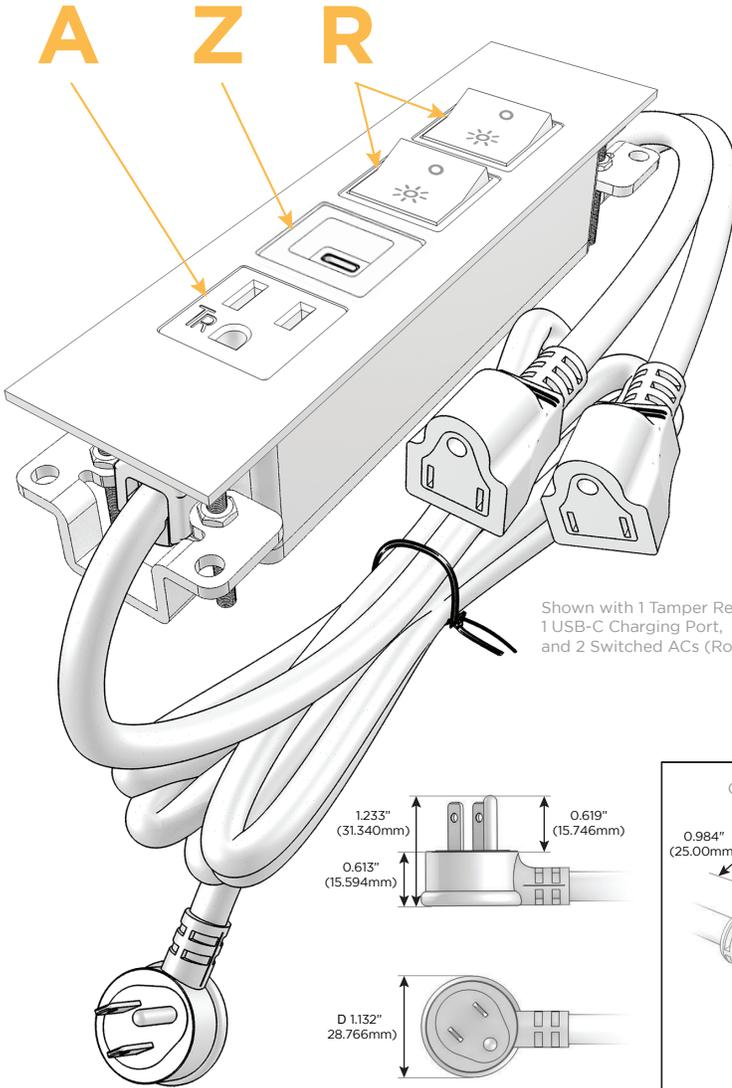
Shown with 1 Tamper Resistant AC, 1 USB-C Charging Port, and 2 Switched ACs (Rocker Switches).
