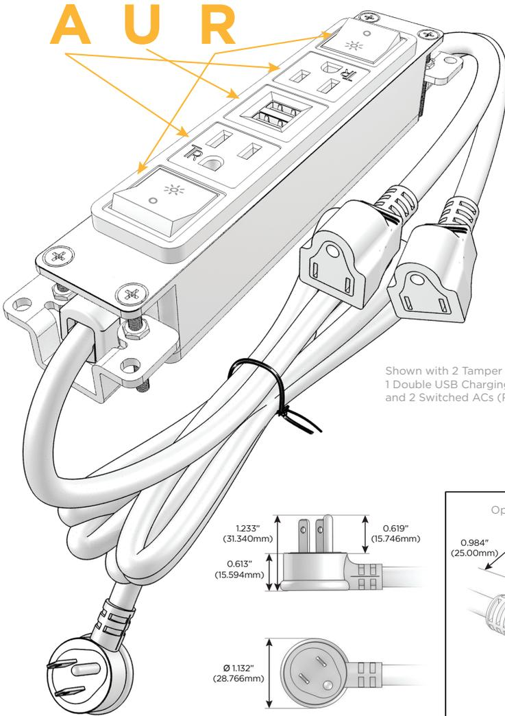
Shown with 2 Tamper Resistant ACs, 1 Double USB Charging Port, and 2 Switched ACs (Rocker Switches).
