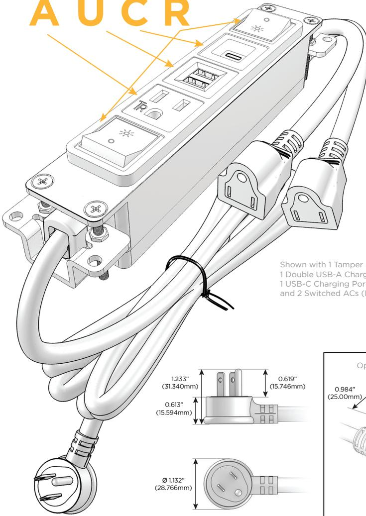
Shown with 1 Tamper Resistant AC, 1 Double USB-A Charging Port, 1 USB-C Charging Port, and 2 Switched ACs (Rocker Switches).
