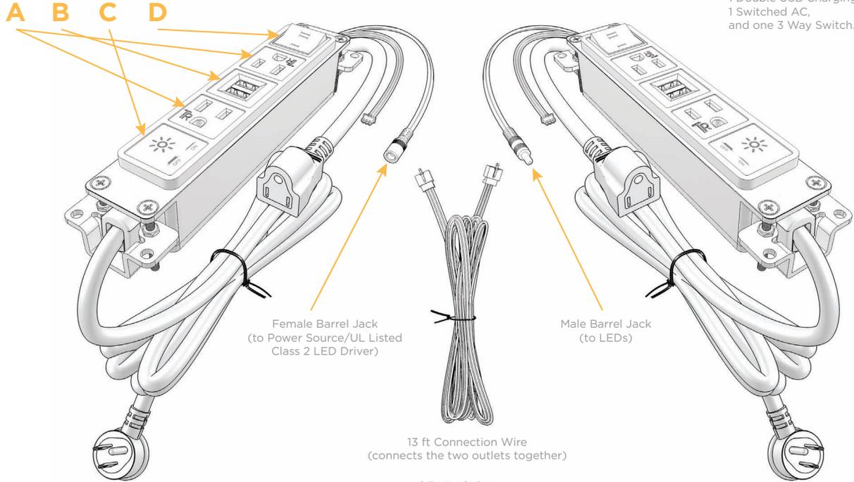
Shown with 2 Tamper Resistant ACs, 1 Double USB Charging Port, 1 Switched AC, and one 3 Way Switch.
