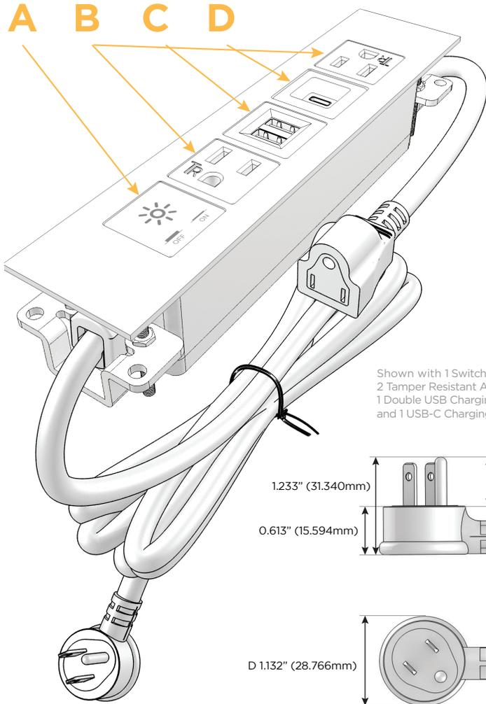
Shown with 1 Switched AC, 2 Tamper Resistant ACs, 1 Double USB Charging Port, and 1 USB-C Charging Port.
