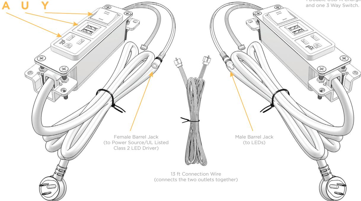
Shown with 1 Tamper Resistant AC, 1 Double USB-A Charging Port, and one 3 Way Switch.
