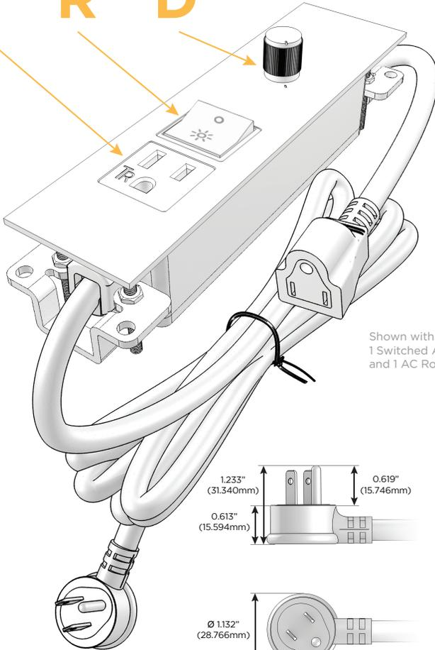
Shown with 1 Tamper Resistant AC, 1 Switched AC (Rocker Switch), and 1 AC Rotary Dimmer Switch.
