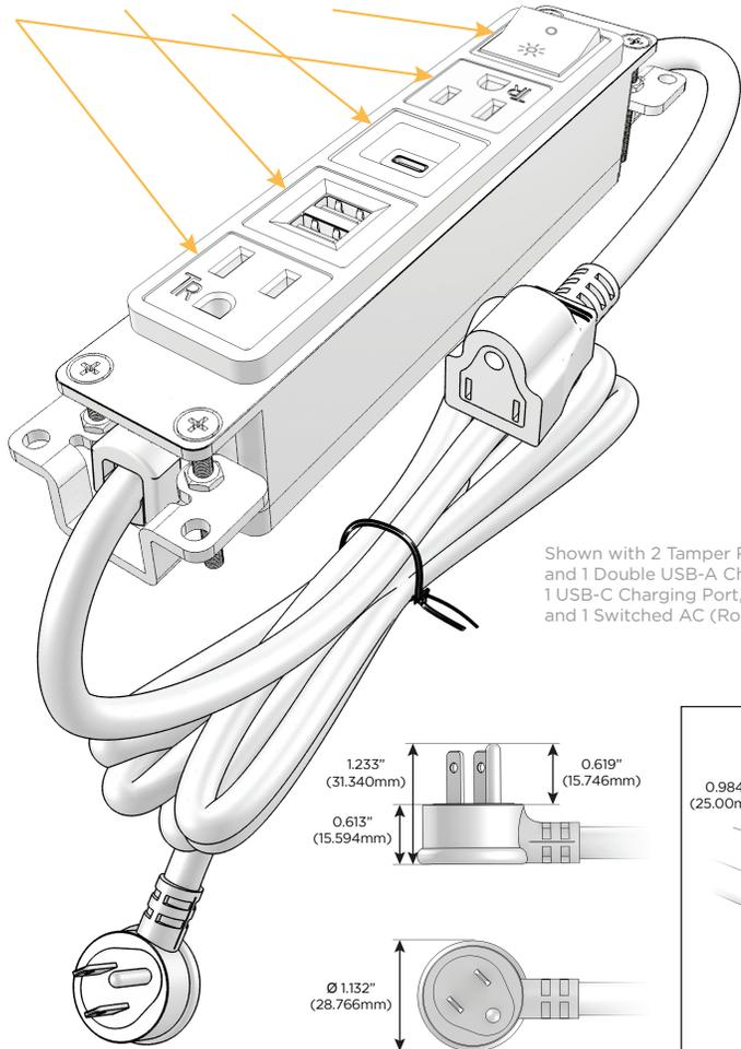
Shown with 2 Tamper Resistant ACs, and 1 Double USB-A Charging Port, 1 USB-C Charging Port, and 1 Switched AC (Rocker Switch).
