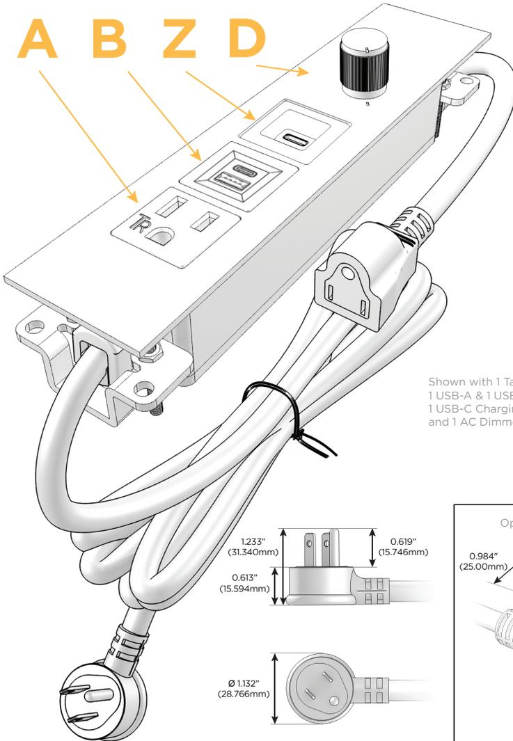
Shown with 1 Tamper Resistant AC, 1 USB-A & 1 USB-C Charging Port, 1 USB-C Charging Port, and 1 AC Dimmer.
