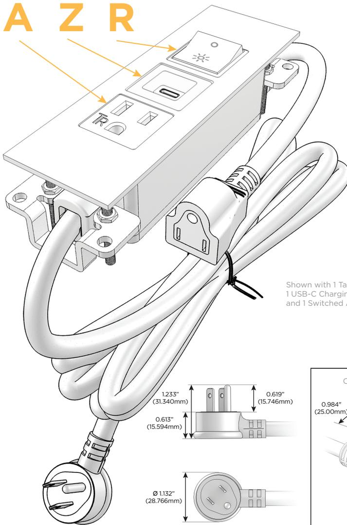
Shown with 1 Tamper Resistant AC, 1 USB-C Charging Port, and 1 Switched AC (Rocker Switch).
