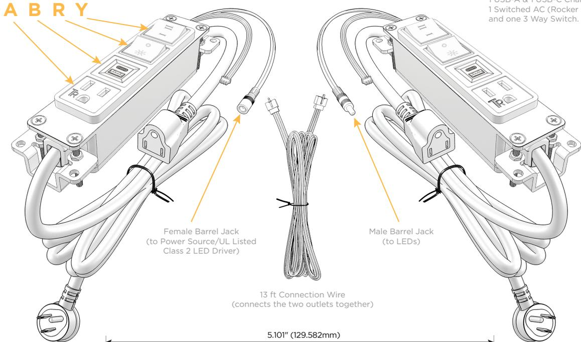
Shown with 1 Tamper Resistant AC, 1 USB-A & 1 USB-C Charging Port, 1 Switched AC (Rocker Switch), and one 3 Way Switch.
