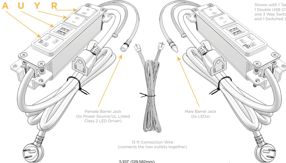
Shown with 1 Tamper Resistant AC, 1 Double USB Charging Port, one 3 Way Switch, and 1 Switched AC (Rocker Switch).
