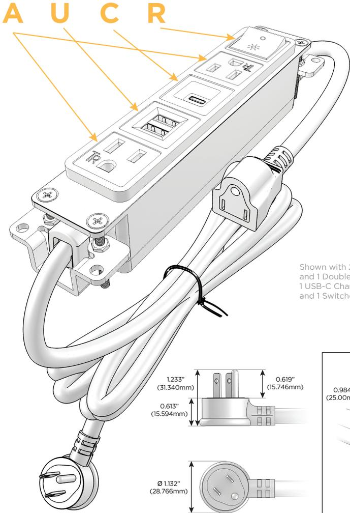
Shown with 2 Tamper Resistant ACs, and 1 Double USB-A Charging Port, 1 USB-C Charging Port, and 1 Switched AC (Rocker Switch).
