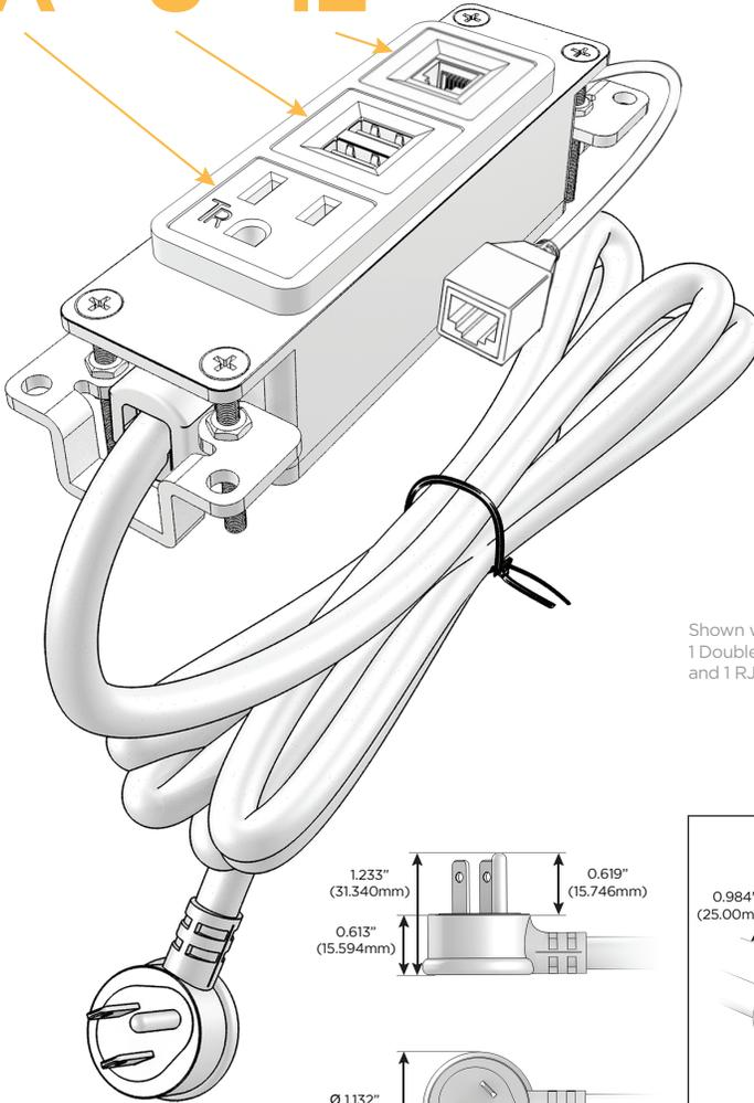
Shown with 1 Tamper Resistant AC, 1 Double USB-A Charging Port, and 1 RJ 12 Port.
