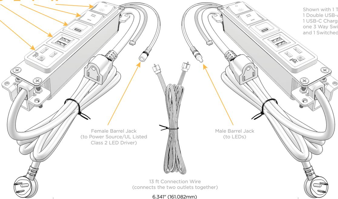
Shown with 1 Tamper Resistant AC, 1 Double USB-A Charging Port, 1 USB-C Charging Port, one 3 Way Switch, and 1 Switched AC (Rocker Switch).
