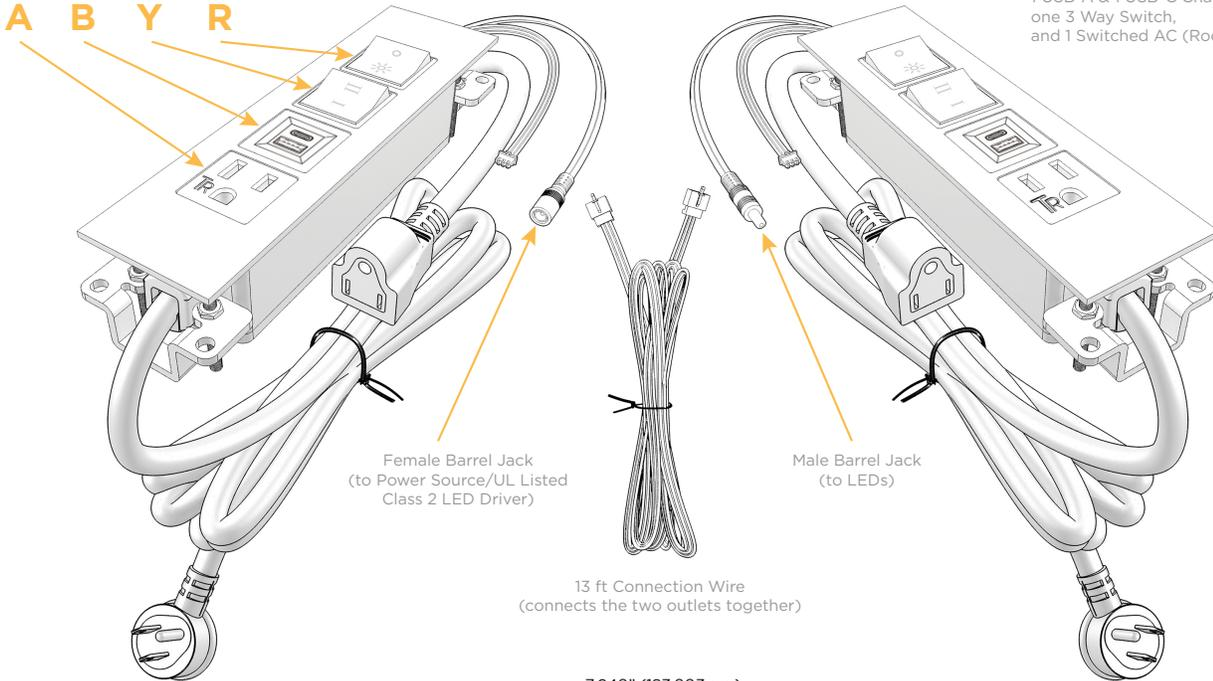
Shown with 1 Tamper Resistant AC, 1 USB-A & 1 USB-C Charging Port, one 3 Way Switch, and 1 Switched AC (Rocker Switch).
