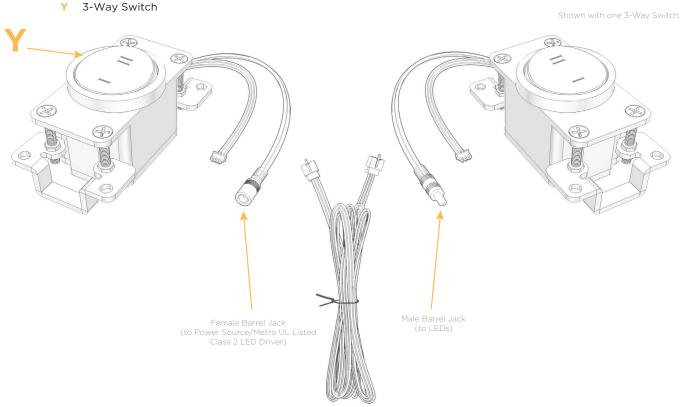
13 ft Connection Wire (connects the two outlets together)
