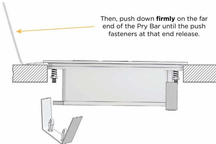
Then, push down **firmly** on the far end of the Pry Bar until the push fasteners at that end release.
