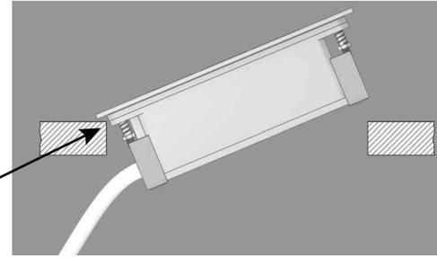
Mounting Clips compress to fit through hole.
