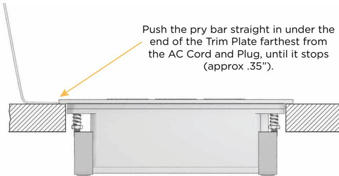
Push the pry bar straight in under the end of the Trim Plate farthest from the AC Cord and Plug, until it stops (approx .35").
