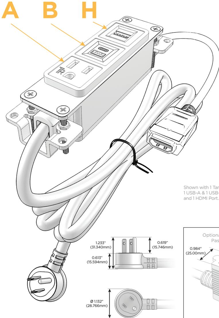
Shown with 1 Tamper Resistant AC, 1 USB-A & 1 USB-C Charging Port, and 1 HDMI Port.
