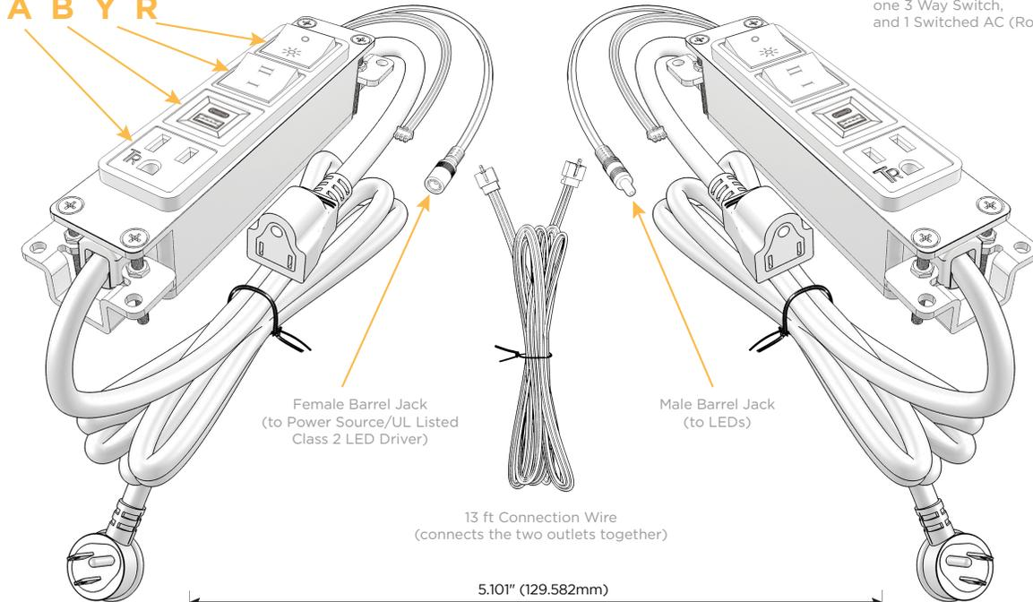
Shown with 1 Tamper Resistant AC, 1 USB-A & 1 USB-C Charging Port, one 3 Way Switch, and 1 Switched AC (Rocker Switch).
